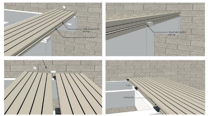
Please refer to installation guides for expansion tables, it is very important to adhere to expansion and contraction guidance when installing composite materials.
